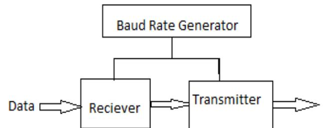
UART communication module is actually the realization of the three sub-modules. The baud rate generator is used to produce a local clock signal which is much higher than the baud rate to control the UART receive and transmit; The UART receiver module is used to receive the serial signals at RXD, and convert them into parallel data; The UART transmit module converts the bytes into serial bits according to the basic frame format and transmits those bits through TXD.
