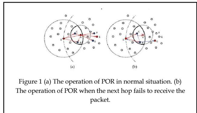
Figure 1 (a) The operation of POR in normal situation. (b) The operation of POR when the next hop fails to receive the packet.
